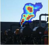
project will investigate using gas imaging cameras for identifying and detecting leaks on buried piping systems as well as other gas facilities.
